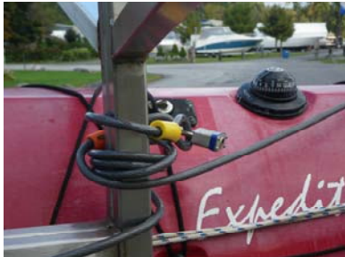
Left to right, Figures 5, 6 & 7. Cables wrapped around the racks upright and padlocked together (fig 5). Padlock loop correctly toward back of boat (yellow cable bumper) nearest the rack upright (fig 6) and padlock loop incorrectly near center of boat (orange cable bumper).
