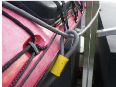
Left to right, Figures 5, 6 & 7. Cables wrapped around the racks upright and padlocked together (fig 5). Padlock loop correctly toward back of boat (yellow cable bumper) nearest the rack upright (fig 6) and padlock loop incorrectly near center of boat (orange cable bumper).
