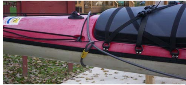
Figures 3 & 4 Make a loop and slip it over the end of the boat. Avoid being too close to the end or near the widest part of the boat.
